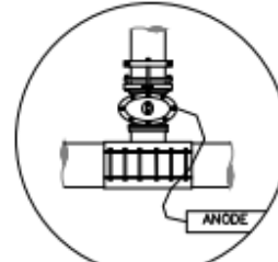
7.7 kg ANODE FOR EACH TAPPING SLEEVE AND VALVE WITH RESTRAINT ASSEMBLY OVER 80 mm Ø, ALL OTHERS TO BE PROTECTED WITH A 2.7 kg ANODE.
